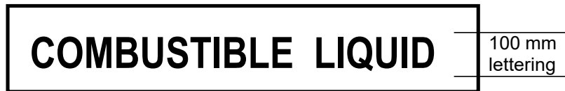
Figure 13.5 Placard for flammable liquid category 4
