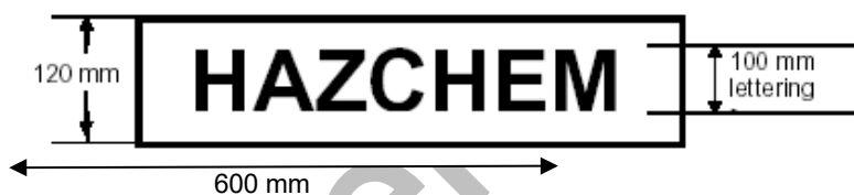
Figure 13.1 Form and dimensions of outer warning placard
