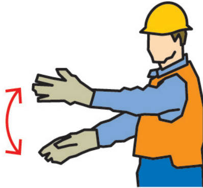
SLACK THE HAULBACK Hands on front of the body using chopping motion
