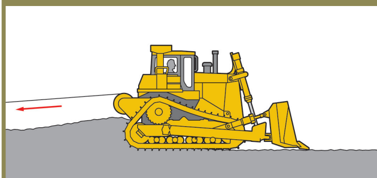
FIGURE 13 A bulldozer used as an anchor point
