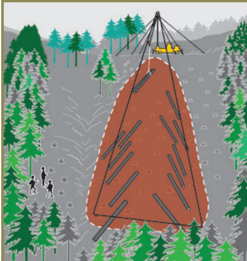
FIGURE 31 Standing in a safe area while logs are being yarded
